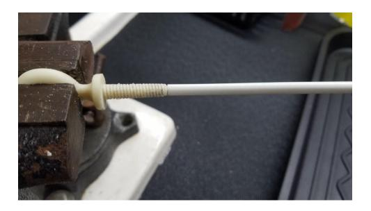
Then I spiral-wrapped a fiberglass cloth strip soaked in epoxy over the joint and built it up for strength. The result was sanded smooth and appeared to be very strong.
